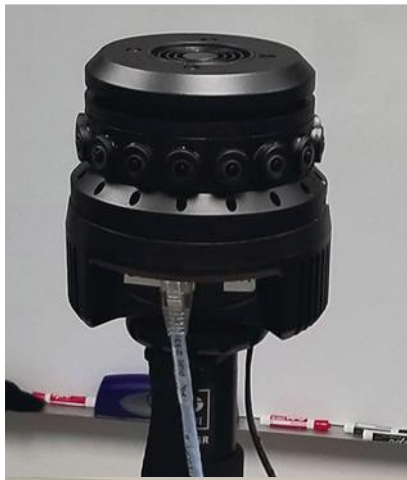
Live Planet's virtual-reality 360-degree camera for video conferencing uses NVIDIA's Jetson TX2 to knit video streams from 16 4K cameras.
