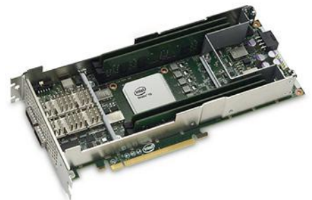
5. Intel's PSG Stratix 10 employs a Stratix 10 FPGA based on the company's Hyperflex FPGA architecture.
