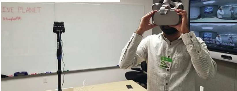
Live Planet's virtual-reality 360-degree camera for video conferencing uses NVIDIA's Jetson TX2 to knit video streams from 16 4K cameras.
