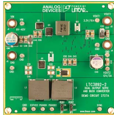
Figure 4. Demonstration Circuit DC2727A. The LTC3892 Controls Two Outputs, a Non-Coupled SEPIC and a Step-Down Converter. [[ V_{IN} 6V-40V, V_{OUT1} 3.3V at 10A and 12V at 3.0A.]]
